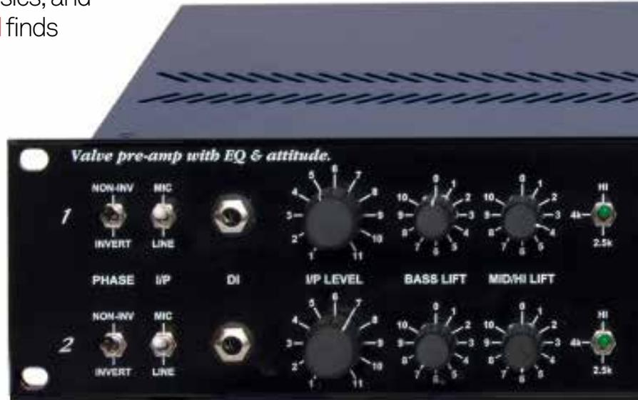
unit. At the lowest Attitude setting, the unit provides 56dB of clean mic gain, which is plenty for any microphone, including insensitive designs such as our Coles 4038 ribbon mic.
