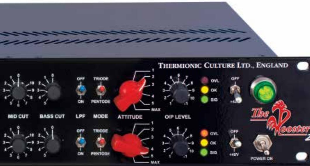
pots that control Bass Lift, Mid/Hi Lift and Mid Cut, along with a six-position rotary switch for Bass Cut. This EQ is a joy to use, providing a powerful range of EQ curves that shape flat signals in a sonically flattering way. It's not a forensic tool for taming nasty frequency spikes – parametric or graphic EQs are better suited to that task – rather, it's a superb tone enhancer designed to bring out the best in both individual sound sources and stereo mixes.
